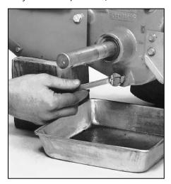
Figure 5-3: Remove drain plug to drain transmission gear oil (also remove oil fill plug and oil level check plug).
